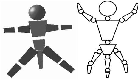
Figure 3: Kinematic structure of a CG model with bend-able limbs with 12 joints and 24 DoF
